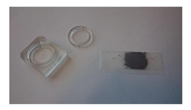
Once you have wrapped your sample into a PARAFILM foil, you can put it inside of sample container – and then into the sample chamber. Now, you can start measurement.
