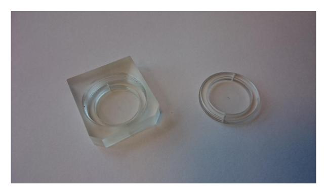
If you are using powder samples, it is smart to wrap them into a thin foil. We are usually using **PARAFILM** foil (it is possible to use even ordinary paper).
